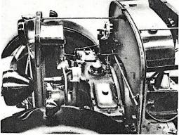
Top—Installation of a Diesel engine in this 1½-ton truck resulted in one-eighth cent per mile operating costs. Lower—Closeup showing the compact 2-cylinder Diesel engine used.
