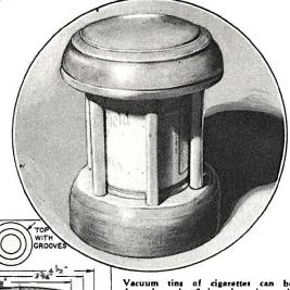
Vacuum tins of cigarettes can be dressed up by fitting them in small dowel containers like the one pictured above. Turn discs from birch or gum. Dowel rods support the assembly. A celluloid liner hides the can.
