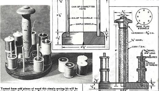
Turned from odd pieces of wood this simple sewing kit will be welcomed by the homemaker. Base is provided with dowels for holding 16 thread spools. Pins and needles are stuck in cord handle. Handle is wood dowel over which carks are glued.
