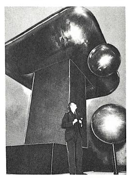
Dr. John G. Trump examines the million-volt electrostatic generator he developed for a Boston hospital. It operates giant X-ray tube to provide radiations for cancer treatments.
