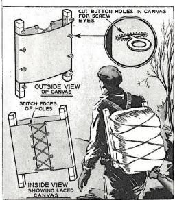
Screw-eyes mounted along the uprights permit the pack to be fastened firmly in place with leather thongs. To ease carrying, a canvas back is attached over frame and laced as shown.
