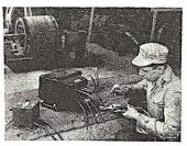
Designed for sweat-soldering pipes and Designed for sweat-soldering pipes and other metal articles these welding pliers are single hand operated. A heavy duty transformer carrying a low voltage-high amperage current heats the electrodes.
