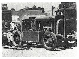
Made from salvaged auto parts this mobile electric welder was built by D. D. Fowble, an Alhambra, Calif., garage operator. It extends his working range to include entire state.
