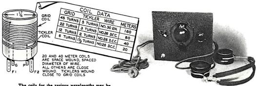
The coils for the various wavelengths may be wound on 4-prong tube bases if commercial coils are not available. If the set fails to oscillate reverse the coil leads P and F-2.
