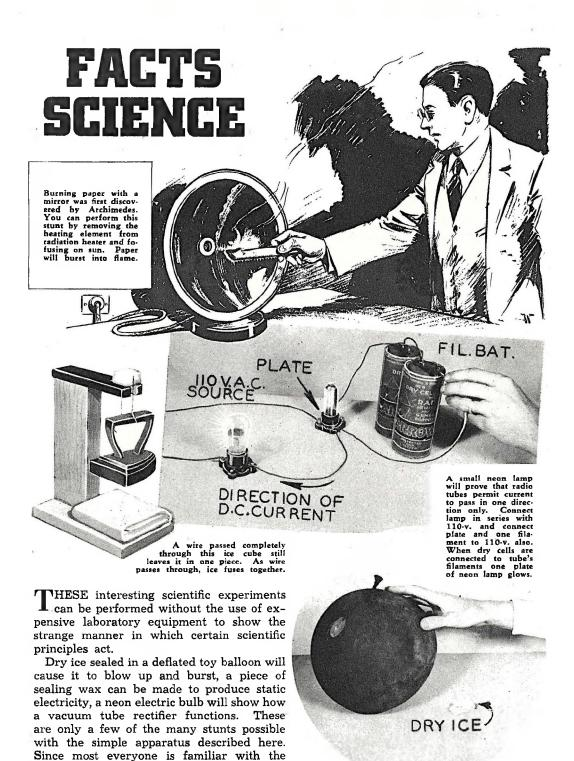
A toy balloon in which several pieces of dry ice have been placed will expand until it bursts if neck is closed. Stunt demonstrates how gas expands when changed from solid to vapor.
