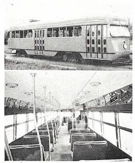
Top—Exterior view of the new electric car developed by Electric Railway Presidents' Conference Committee. They start and stop quicker, can speed at 50 m.p.h., and are fitted brakes-dynamic, magnetic and air. Bottom-Interior view of the car showing the seating arrangement
