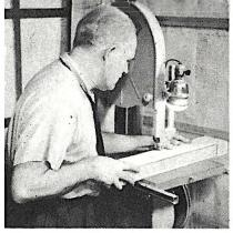
The runners are cut out on a band saw from maple, oak or No. 1 pine. The sawing operation is shown in the above photo. The plan shown at right gives the necessary runner dimensions. Runner shoes are cut from ½" by 2" C. R. steel.
