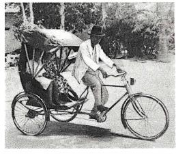
Pedaled like a bicycle, this new type rickshaw has speeded up street transportation in British Malaya. Invented by a Chinese, the odd locking vehicle replaces the old hand pulled rickshaw.
