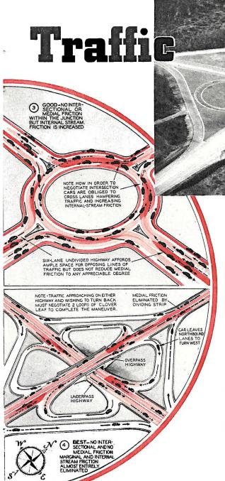
Though theoretically traffic flow never ceases in rotary junction (upper right) there is still danger and delay. Cloverleaf juncture of two roads with median strips (lower right) is traffic at its best. There is no congestion, little delay.
