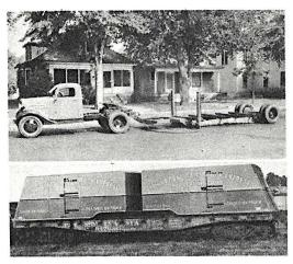
Top—This trailer chassis can be raised or lowered by compressed air device on truck. Bottom—Trailer bodies can be set flush on floor of railroad flatter, eliminating topheaviness in transit, enabling locomotive to maintain speed along route.
