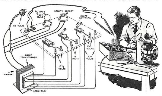
This electrical test panel is a useful piece of equipment for the radio or electrical experimenter's workbench. It can be built from parts salvaged from a junked receiver if new materials are not available for the purpose. A 300-volt transformer provides plate and filament voltages for experimental circuits. Neon lamp connected across 110-volt leads is handy point-to-point tester.
