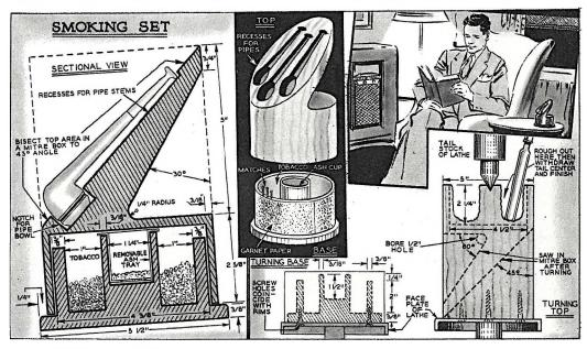
Not only is this Smoking Set an attractive home workshop project but a useful article for the den as well. Several different kinds of contrasting hardwoods glued up into a block will provide a unique turned lathe article. The tobacco compartment holds a full can of smoking mixture. The top of the Smoking Set serves as a pipe rack. Three pipes conveniently fit into lid.
