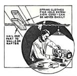
Spring clothes pins attached to the walls and ceiling of workshop are useful for holding extension cords.
