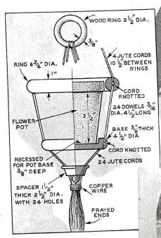
Turned on a lathe from scrap pieces of gum this hanging plant basket proves a novel home decoration. The above diagram gives the cross-section details.
