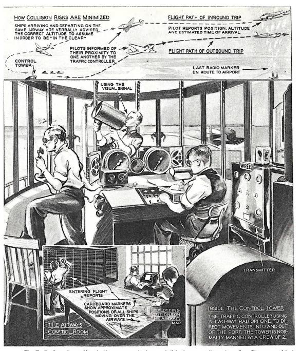
The Traffic Controller at Newark Airport uses radiophone and light beams to direct air traffic. Planes are advised when to land or take off. Pilots without radio equipment are advised by red or green light beams directed at plane.
