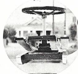
This front-end view shows the steering gear assembly. The steering shaft is held rigidly erect by a length of  $1\frac{1}{2}$ -inch pipe and a floor flange mounted on top of chassis board. Steering wheel connects to front runners through universal joint disc.
