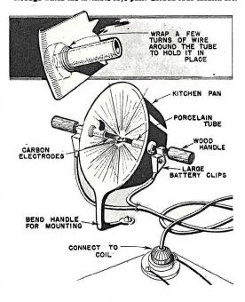
A pair of carbon electrodes or rods of \( \frac{3}{6} \)" dismeter connected to the reactance coil and fitted in a reflector similar to the one shown here make a powerful spotlight. Porcelain insulators such as used in house wiring insulate carbons from reflectors.
