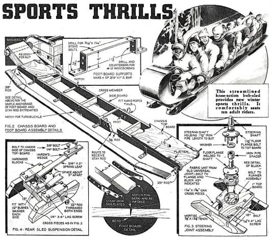
to rock through an angle of about fifteen degrees without the slightest lost motion, or lash, in the steering shaft itself. The parts needed for this can be picked up at any auto wrecking yard for a few cents.
