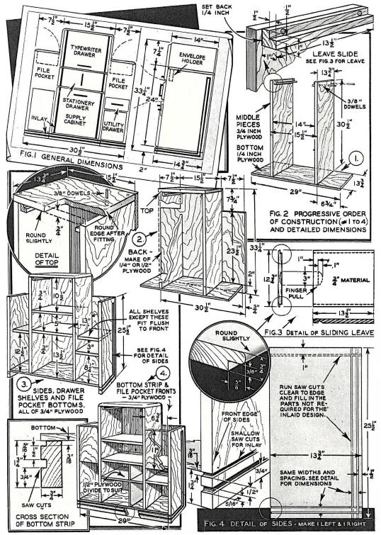
General cabinet dimensions of the deak are covered in this diagram. On all joints where stress will be placed dowel pins should be used. Careful assembly will result in a workshop project that will equal many commercial deaks of similar design.
