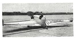
Steered by rudders placed at each wing tip, this tailless monoplane piloted by Prof. John D. Akerman, of the University of Minnesota, is said to have excellent flying qualities.
