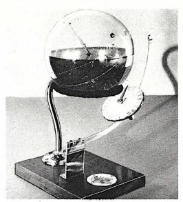
This astroglobe has 24 constellations marked on it. Device rotates every 24 hours to represent motion of celestial bodies around the earth, imagined to be at exact center of globe.
